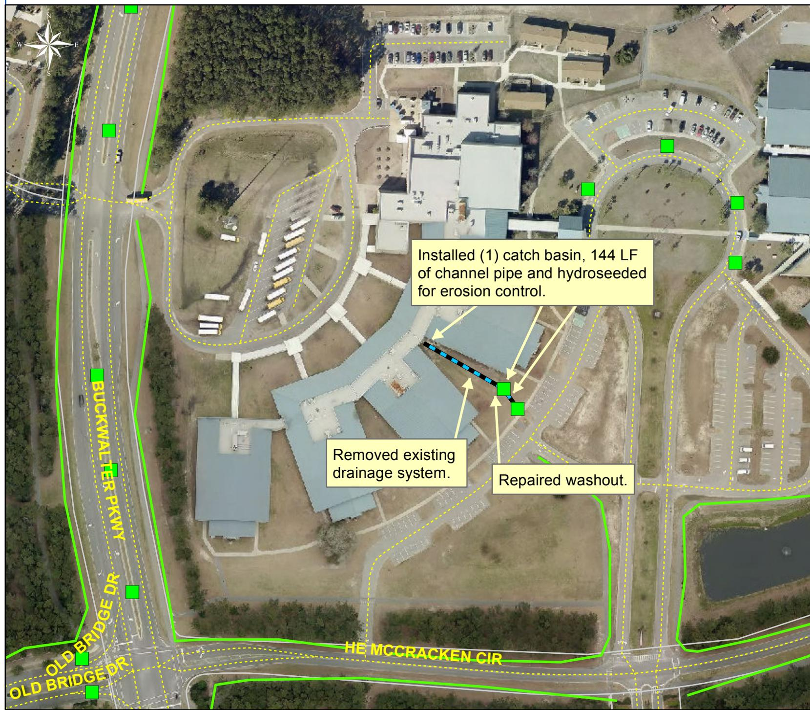
Installed (1) catch basin, 144 LF of channel pipe and hydroseeded for erosion control.
